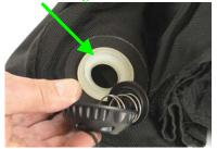
Wrong! Gasket placed in Exhaust Valve connection
